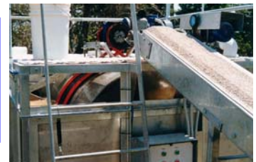
Above: HALT system dosing into Partridge creek. Right: Delivery of lime from hopper to HALT system.
