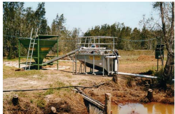
Above: HALT system dosing into Partridge creek. Right: Delivery of lime from hopper to HALT system.
